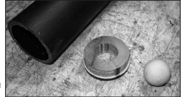
The top cap is simply there to keep the piston rod aligned with the pump body.
