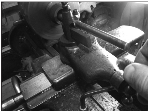
Boring inside taper with compound set at 84°
