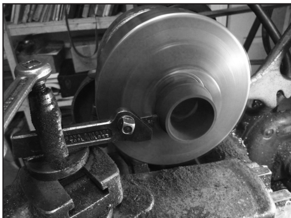
Parting. Tool extended to avoid interference with chuck.
