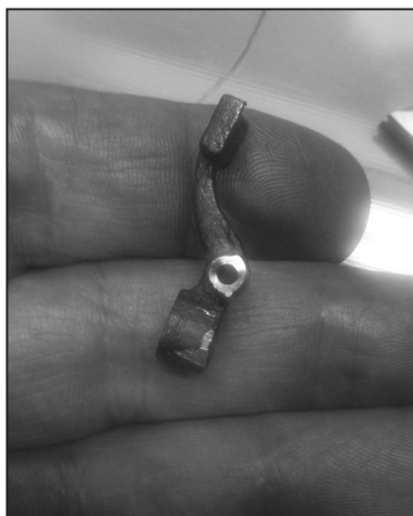
A newly machined float arm pivot hole.
