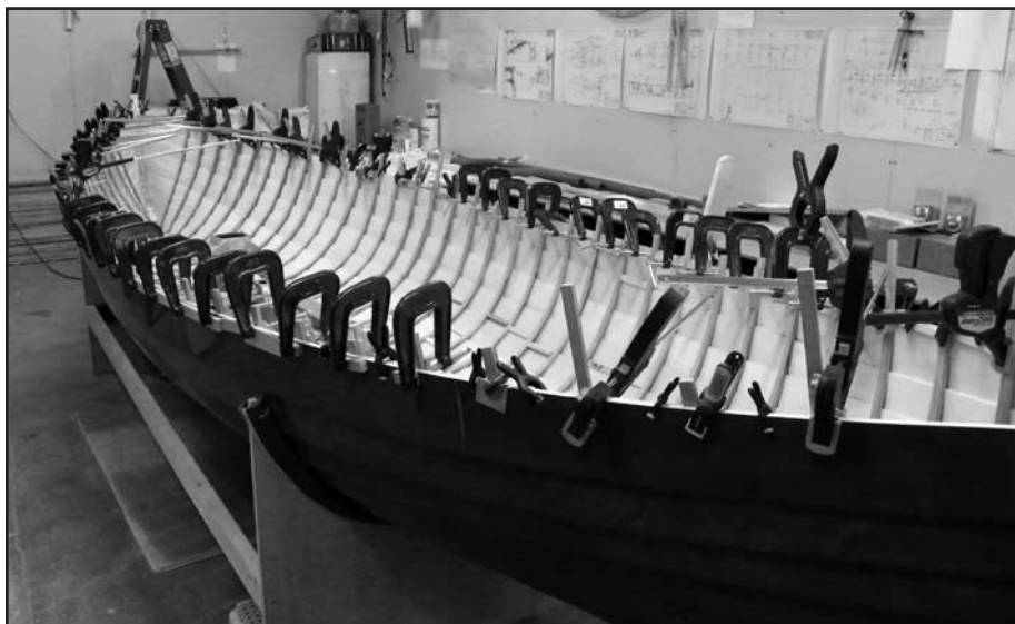
Clamps, clamps and more clamps. Can you ever have enough when you build a boat?
