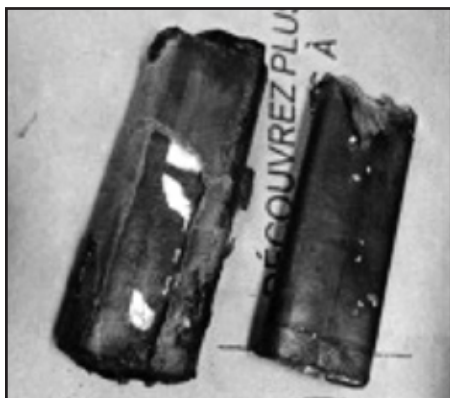
Two original shorted capacitors showing waxed paper and tin foil.
