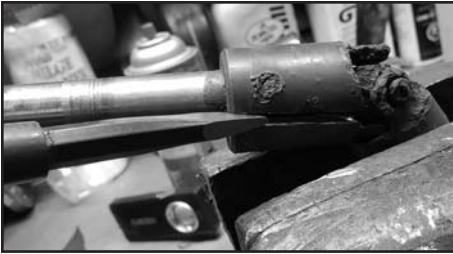
Delicate work with a zip cut wheel and chisel to split the old joint off the shaft.
