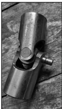
Sliding pin type u-joint with small pin coming out. What could go wrong?
