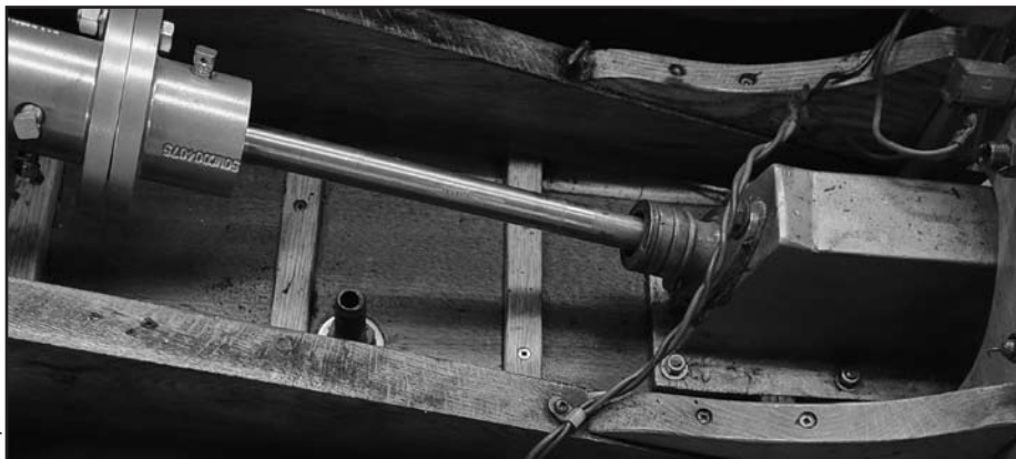
Checking that the shaft is centred in the device hole before installing the stuffing box.
