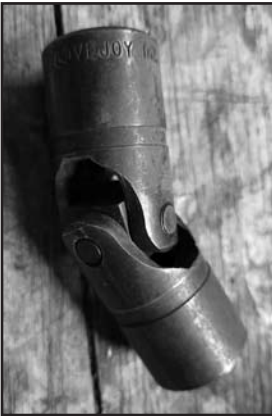
Pin and block type u-joint. Notice the pins are all the same size.
