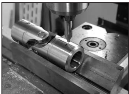
Drilling and tapping the holes in the new universal to match the shaft.
