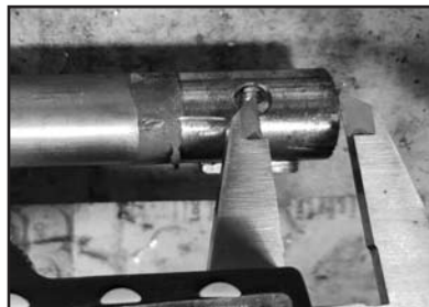
Measuring to drill new grub screw holes that match the dimples
