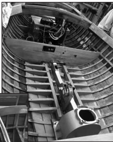
From the Stern; everything is in the engine room or under the seats except the lever by the device which is the single lever control, Forward, Neutral, Reverse and Throttle combined.
