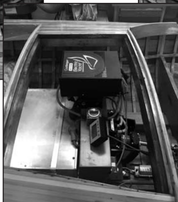
Amidships; rear of battery, Electric Yacht motor controller and beneath that the motor.
