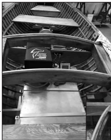
From the bow; the aluminum box is the 'all day' battery.
