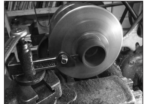
Parting. Tool extended to avoid interference with chuck.
