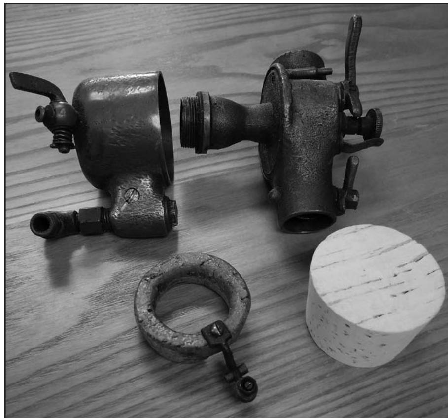
The finished float for the Kingston Four Ball and the raw material from which it was manufactured.
