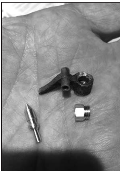
The project so far. A new brass needle, a new nut and the old broken float arm used as a thread gauge. Not only does it all fit, but once assembled, it all articulates in the arm as it should.
