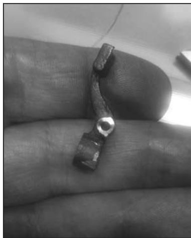
A newly machined float arm pivot hole.
